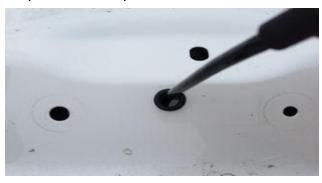
**Step 5:** Route camera and/ or chassis harness along existing wiring and secure using wire ties or electrical tape. IMPORTANT: Ensure harnesses move freely with the trunk or liftgate.
