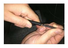
**Step 7:** Route chassis harness forward. It may be necessary to remove sill plates, pillar covers, side panels, etc. Use a plastic trim removal tool to avoid damage to trim pieces.
