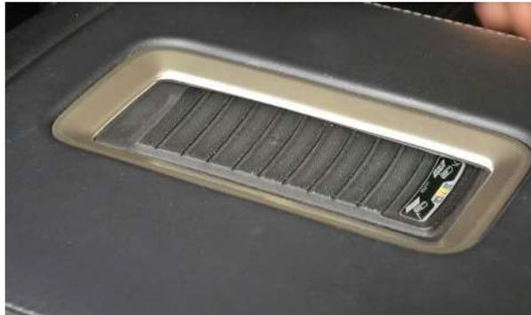
6. Reinstall mat retaining Torx Screws. On some models, you may only be able to install 6 of the 7. This will not impair the charger or your console in any way.
