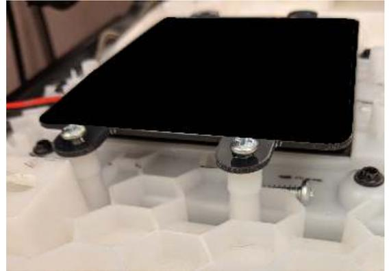
6. Connect power harness to new replacement charging module and snap panel back in place.
