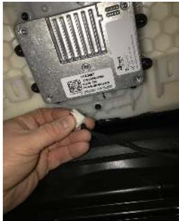
3. Locate 4 screws securing charging module and remove the screws and the charge module. The screws will not be needed for the replacement charger.
