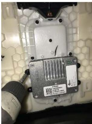
4. **STOP.** Test charger prior to full installation. To accomplish this, connect new power adapter. Set Qi-compatible wireless charging phone directly on charger. Turn key to on position. Phone should begin to charge. Remove power adapter and continue with installation.
