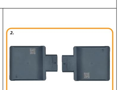
Install Radar units with connector plug facing towards the eachother
