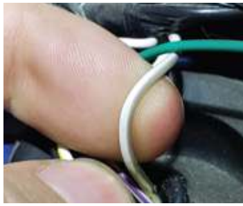
Jeep Wrangler JK 12V Power Location (White/Grey wire by passenger kick panel)
