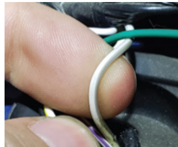
White/Grey 12V Reverse Wire Located in JK Passenger Kick panel
