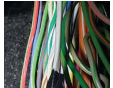
Jeep Wrangler JK 12V Power Location (White/Grey wire by passenger kick panel)
