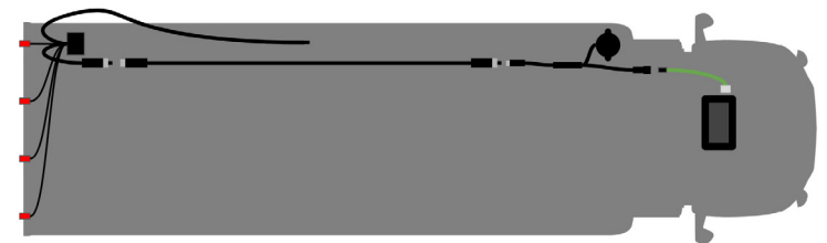
Backup Sensor Wiring
